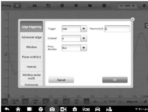
**Figure 7-65 Sample Trigger Settings Screen**
