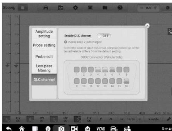
**Figure 7-61 Sample DLC Channel Setting Screen 1**
