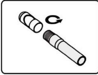
2. Screw the thread part of the accessory over the imager head to fix the accessory.
