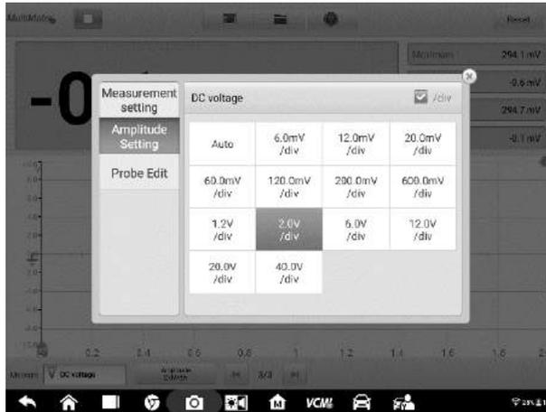
Figure 7-18 Sample Amplitude Setting Screen (DC 2.0V/div)
