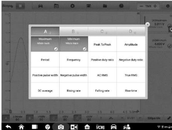
**Figure 7-82 Sample Measurement Setting Screen**
