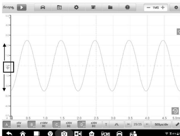
**Figure 7-42 Sample Dragging Zero Baseline Marker Screen**
