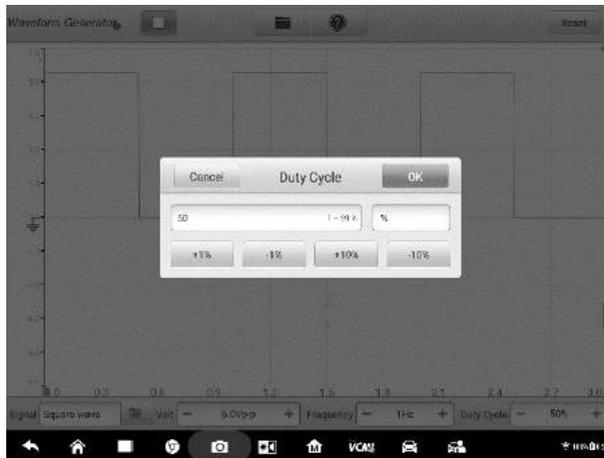
**Figure 7-24 Sample Duty Cycle Setting Screen 2**
