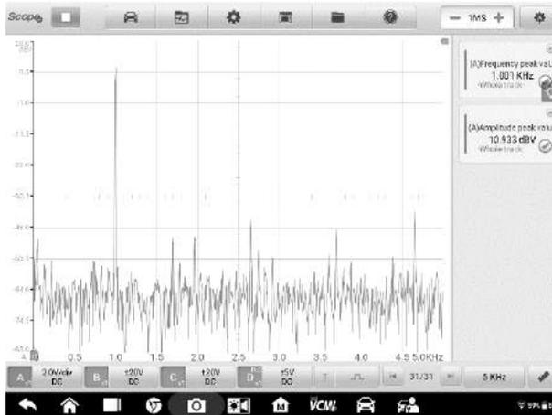
**Figure 7-86 Sample Measurement Display Screen (Spectrum View)**
