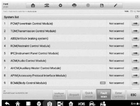
Figure 5-4 Sample Fault Scan on System List Screen
