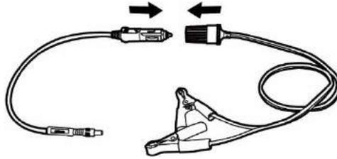
**Figure 4-1 Connection between Cigarette Lighter and Clipper Cable**
