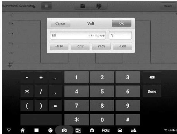
Figure 7-19 Sample Voltage Setting Screen 3
