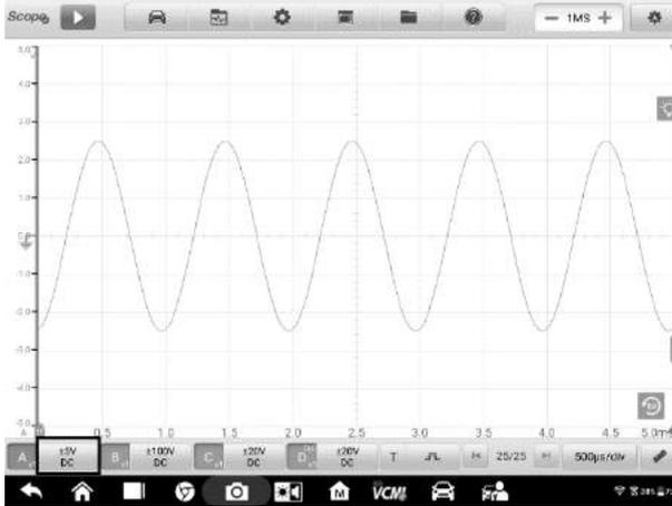
Figure 7-50 Sample Amplitude Setting Screen (DC 5V)
