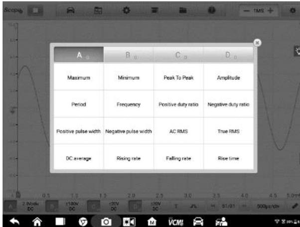
**Figure 7-80 Sample Measurement Screen 1**
