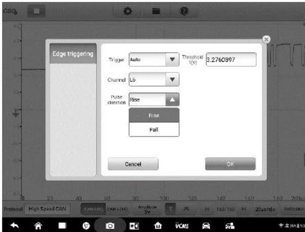
**Figure 7-24 Sample Pulse Direction Screen**
