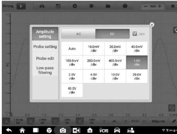
Figure 7-51 Sample Amplitude Setting Screen (DC 1.0V/div)
