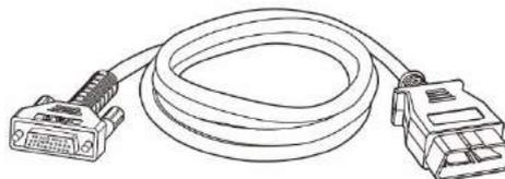
**Figure 2-7 Main Cable – 2 m in length**
