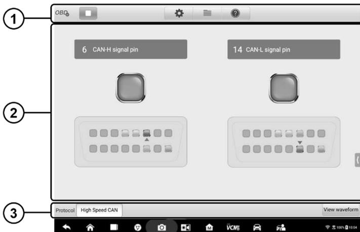
**Figure 7-4 Sample OBDII CAN Bus Check Menu Screen**
